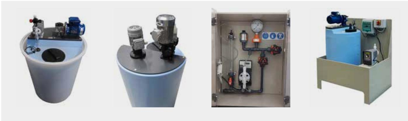
Dosing stations with tanks ranging from 50 to 1000 litres, which can mount an electromagnetic or motor-driven dosing pump, various types of electromechanical or manual stirrers, suction lance with inbuilt level sensor or stilling tube, and safety container.
